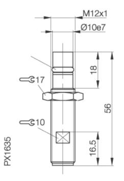
Inductive Sensors BHS B249V-PSD15-S04 M12x1 x 56 normally-open Sn=1,5mm shielded pressure rated to 500 bar
